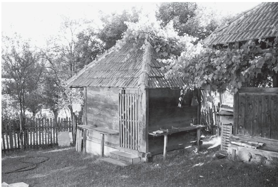
Image 13. A vajat with a frame and an infill of horizontal planks
