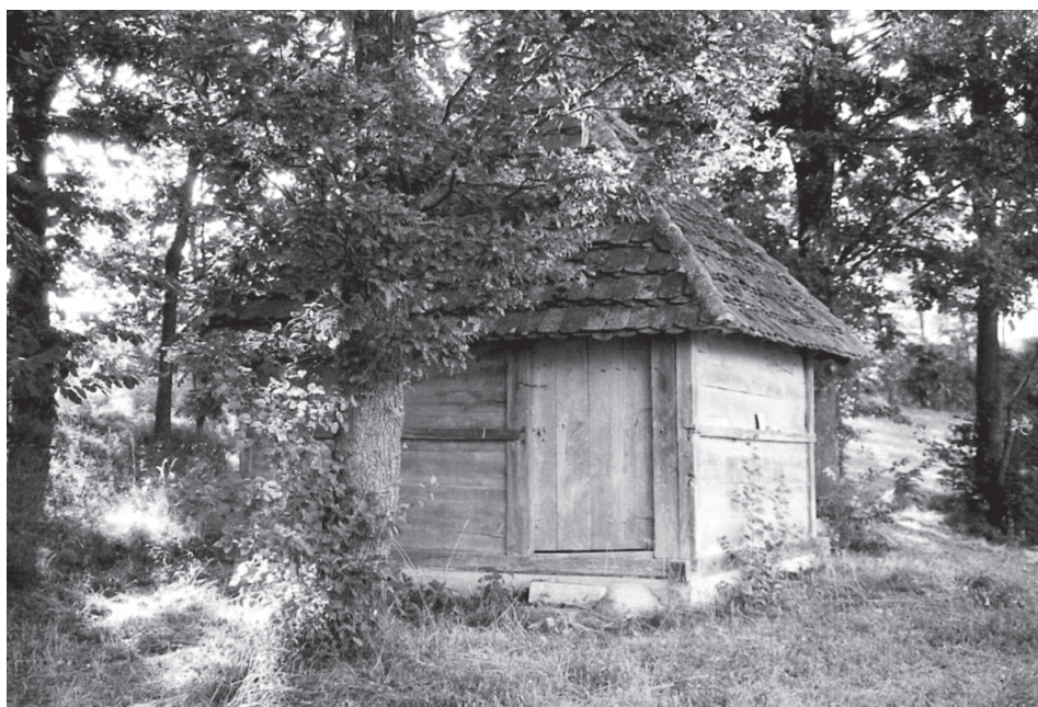
Image 11. A vajat with a frame and an infill of horizontal planks
