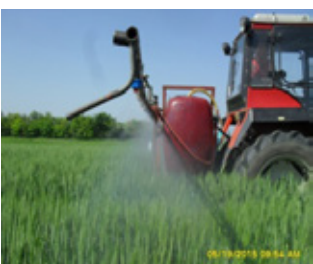
Figure 2. Stream of the nozzle type ATR 8004 (original)
