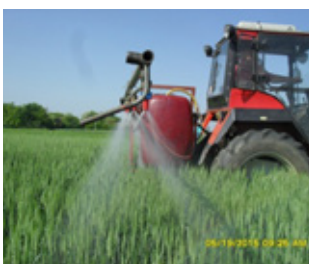
Figure 3. Stream of the nozzle type TFA 11004 (original)
