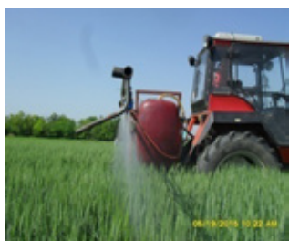
Figure 1. Stream of the nozzle type TJ 11004 (original)
