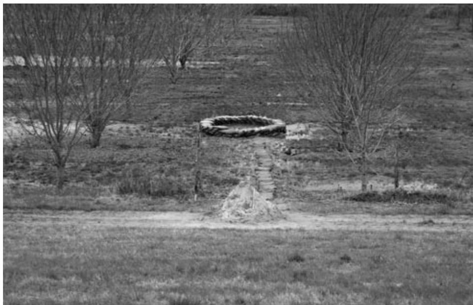
Fig. 3. – Piping at Dombor as seen from the crest of the dyke. Washing out of soil first occurred some 20 meters away from the toe of the embankment (Areas No. 5-8 in Tables 1 and 2)
