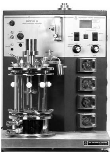
Fig. 1 — BioFlo III fermentor, New Brunswick, with pH and temperature probes
